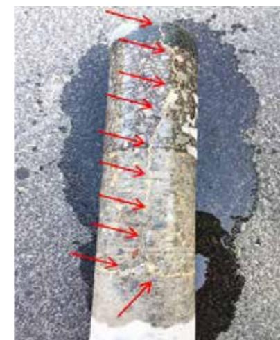
裂缝焊接施工芯样
